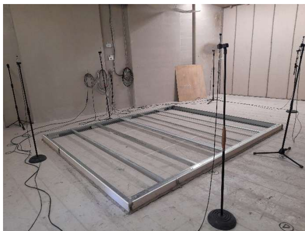
Figure 4_ Reverberation Room Empty with structure
