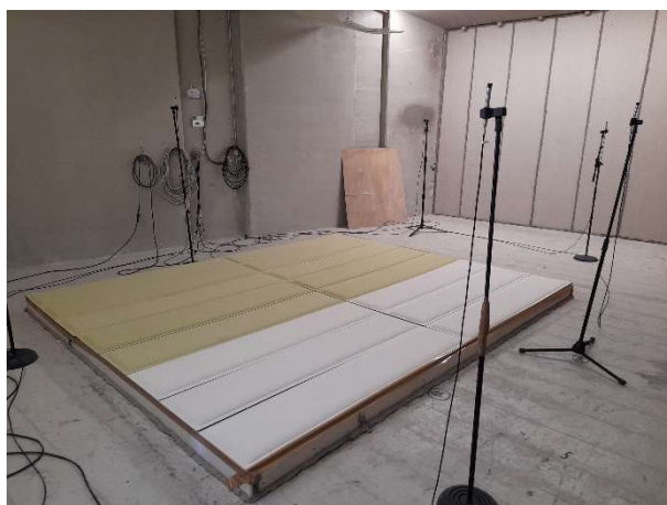
Figure 5_ Reverberation Room with Sample
